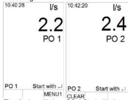
The display will show PO 1.Start with the throttle ring on and press Enter to collect the first value,
