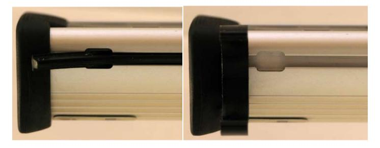
Remove the list by pull it out. When the list has been removed you can place the holders by placing it in the opening and pull them to a suitable place.
