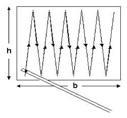
By slowly sweeping (traversing) the sensor above the surface. e.g. an intake grille or the opening to a fume, you measure the total flow. Repeat the measurement until you get the same measure values so that you learn the technique.
