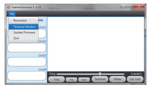
With SwemaTerminal 3 it's possible change settings, print stored measurements, update firmware, print calibration protocol. Information of what kind of instrument and at which COM-port it's connected can be found on the top left side. For SwemaFlow 126 it is only possible to change settings in "Terminal Window".
