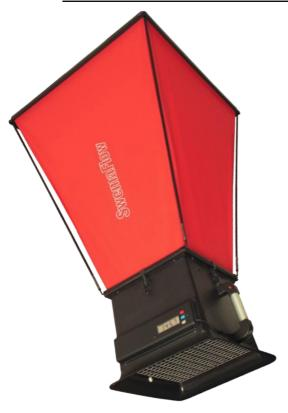
**SwemaFlow 4001** is ideal for testing, adjusting and balancing (TAB) of air flows up to 1500l/s, 3100cfm. SwemaFlow 4001 uses the proven Swema principle, a net of hot wires, which gives a good and accurate mean value for supply and exhaust air flows. Measured values can be stored and transferred to PC.
