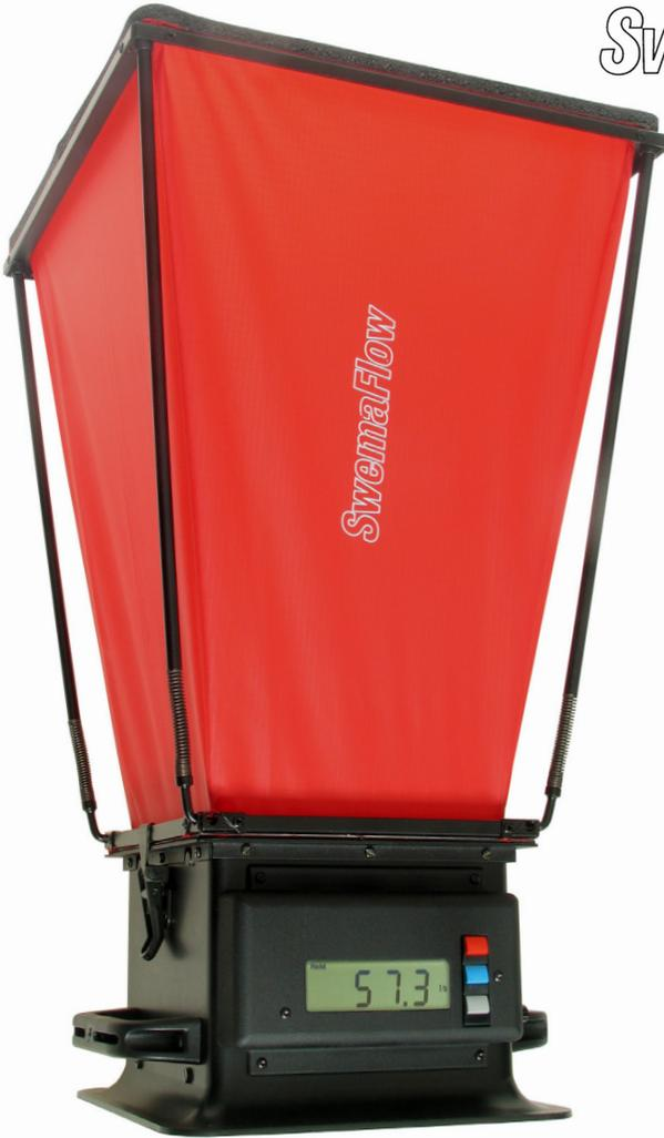
**SwemaFlow 126** is ideal for testing, adjusting and balancing (TAB) of air flows up to 125 l/s, 260 cfm. SwemaFlow 126 uses the proven Swema principle, a net of hot wires, which gives a good and accurate mean value for supply and exhaust air flows. Measured values can be stored and transferred to PC.
